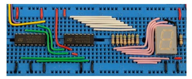
Wiring up the 4511 to a 7 Segment Display and (in this case) 4510 Counter can be challenging using a prototyping board. The photograph shows a good example of how this can be achieved neatly.
