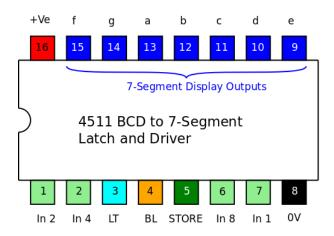
The 4511 accepts a 4 bit Binary input and converts this to the corresponding output to drive a 7 Segment Display.
