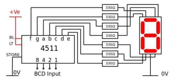
**STORE** is held LOW as it is connected to 0 V. **LT** and **BL** are held HIGH as they are connected directly to the positive supply rail.
