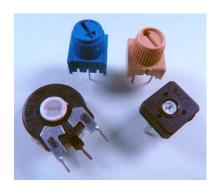
A variable resistor is, as the name suggests, able to have a range of resistances between zero and some stated maximum resistance. Therefore a  $10~\text{k}\Omega$  variable resistor can have any value between  $0~\Omega$  and  $10~\text{k}\Omega$  as determined by the user. Variable resistors are used to control the current in a circuit, an example might be dimming a bulb or slowing a motor or to change time delays or other properties of a circuit.
