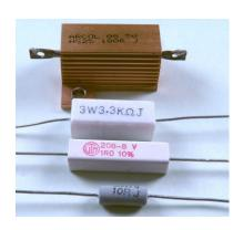
A fixed resistor is, as the name suggests, a fixed predetermined value. Lower power resistors are either made from carbon film or metal film and are the sort of resistor used in timing circuits, analogue circuits, as pull down resistors and to limit low current values in electronic circuits.
