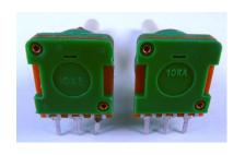
The resistance of a rotary or linear potentiometer can either change linearly with position or logarithmically with position.
