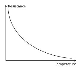
An NTC thermistor is another semiconductor device. The resistance of the semiconductor reduces when thermal energy is supplied. Therefore, the resistance of the thermistor reduces as the temperature increases. This is the usual type of thermistor used in electronics. NTC stands for "Negative Temperature Coefficient" because the resistance goes down as the temperature goes up and vice versa. Thermistors are often used in potential divider circuits to form temperature dependent circuits.
