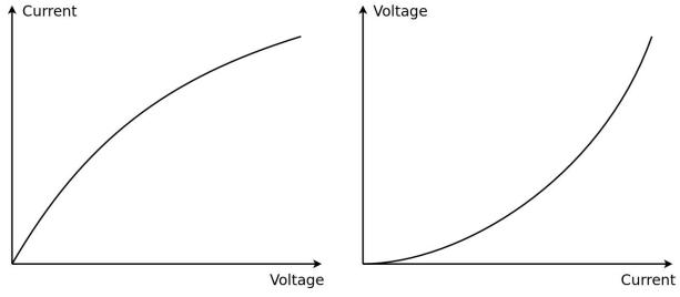
In a resistor such as a hot wire or a filament in a bulb the resistance increases as the temperature increases. The temperature increases because of the current flowing in the conductor. Therefore, in a heating element or filament, the resistance increases as the current and voltage increase. The V-I graph is a curve. NOTE: The gradient of the graph is not the resistance ... this is only true for the special case of an ohmic conductor.
