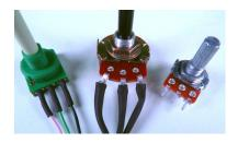
A potentiometer is a much more useful form of variable resistor. In fact a variable resistor is, in reality, a potentiometer with one of the connections remaining unused. A potentiometer has 3 connections.
